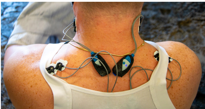
A veteran participant wearing surface electromyography (sEMG) equipment which allowed muscle activity to be recorded during the sessions. These measurements were taken to investigate whether veterans or horses experienced muscular tension (stress) during the sessions.
