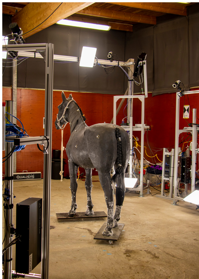
Part of the locomotion laboratory at the Swedish University of Agricultural Sciences. This space is configured for three-dimensional data collection using an optical motion capture system and a 3D scanner. This data will ultimately be used to generate 3D video and data from two-dimensional videos.
